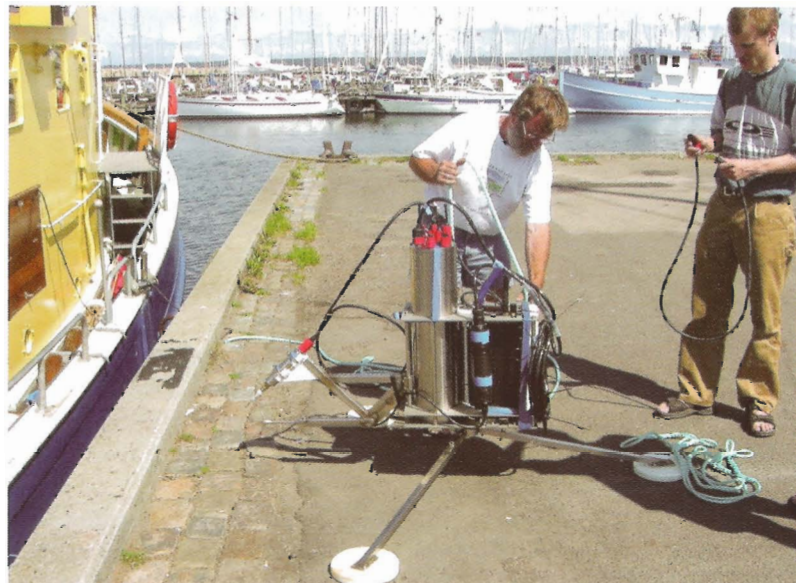
A new instrument conceived by Research Associate Professor Peter Berg will allow researchers to study oxygen depletion on coastal waters more accurately.
